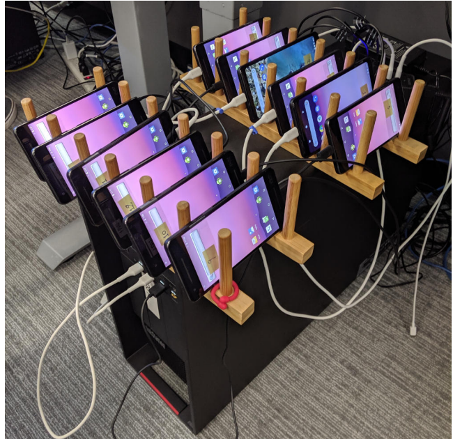
Figure 8: Our device fuzzing cluster.
