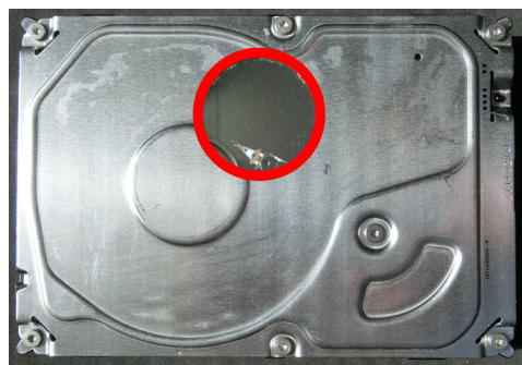
Figure 3: SMR drive with the observation window encircled in red. Head assembly is visible parked at the inner diameter.
