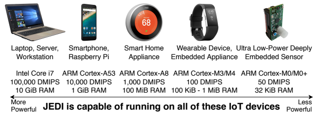
Figure 1: IoT comprises a diverse set of devices, which span more than four orders of magnitude of computing power (estimated in Dhrystone MIPS). 1
